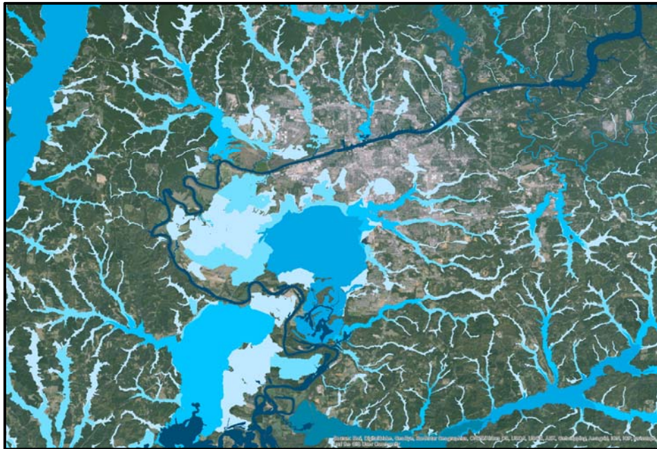
Figure 4. The modified HAND method displaying (from lighter to darker colors) HAND to HAND6 5-meter inundation (there is no flood inundation for HAND7 or HAND8 at this depth). Notice that darker colors shift toward larger streams.
