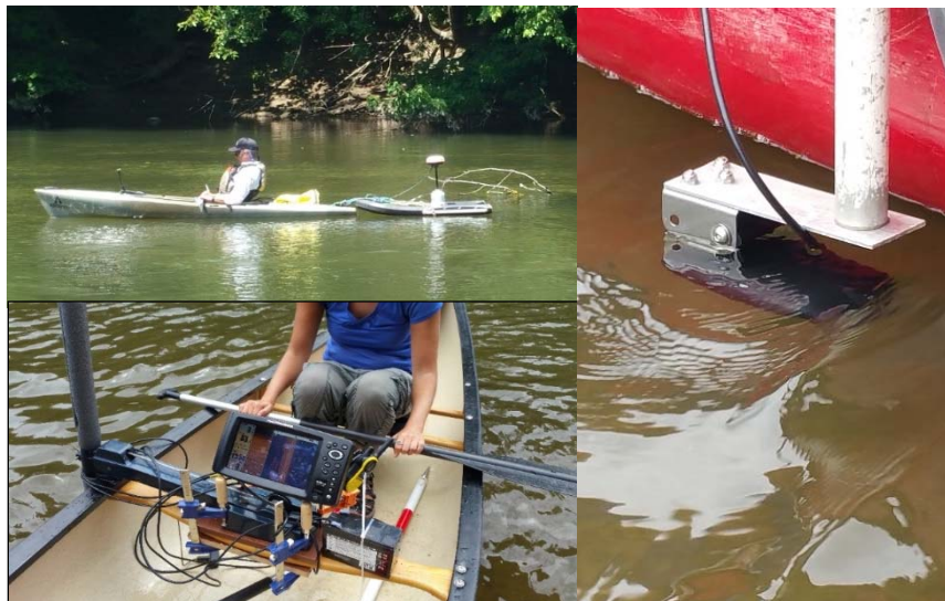
Figure 3. Left: Image of ADCP setup used; Below: Images of the mounting process and orientation of the Humminbird Fish Finder
