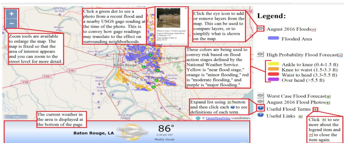
Figure 7. Finalized web interface for Baton Rouge complete with features recommended through the public feedback. Text on the figure explains how to use each map feature. Web map for Dallas (not shown) follows this same framework.
